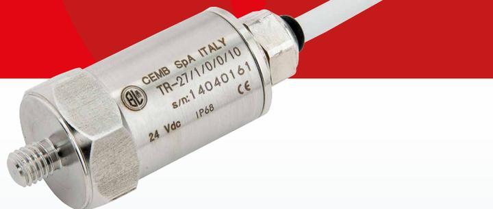
The integrated transmitter TR-27 measures the absolute vibrations of any rotating machine support and it is able to interface directly in 2 wires technique (current loop 4 ÷ 20 mA) to an acquisition system (PLC or DCS).
