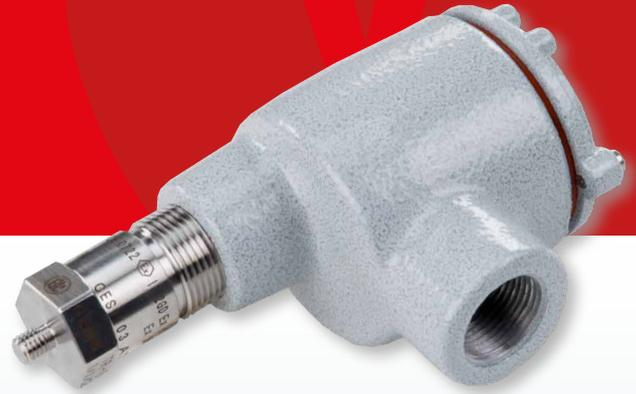
The integrated transmitter TR-I measures the absolute vibrations of any rotating machine support and it is able to interface directly in 2 wires technique (current loop 4 ÷ 20 mA) to an acquisition system. It is made in Explosion proof version for application in aggressive environment.
